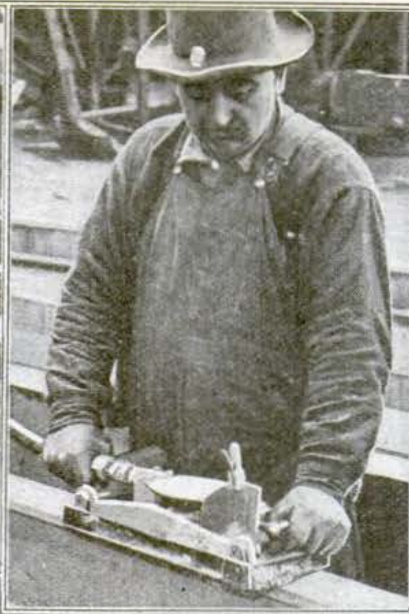
These planers are run by air-driven turbines
