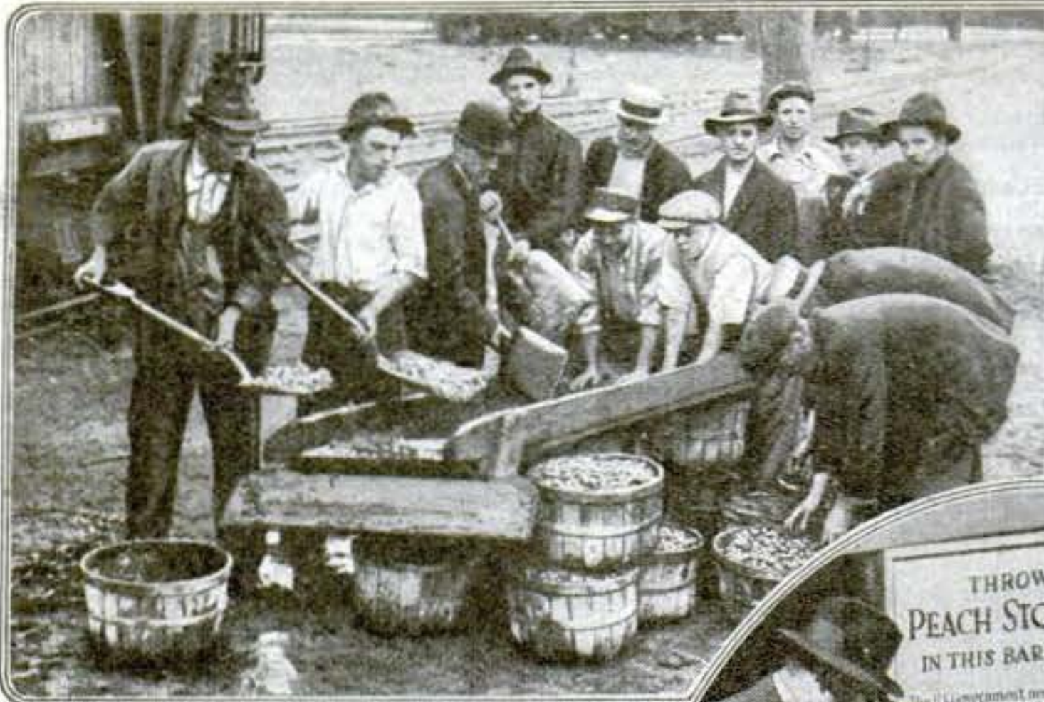
Extracting the stones from peaches as a first step in gas-mask construction
