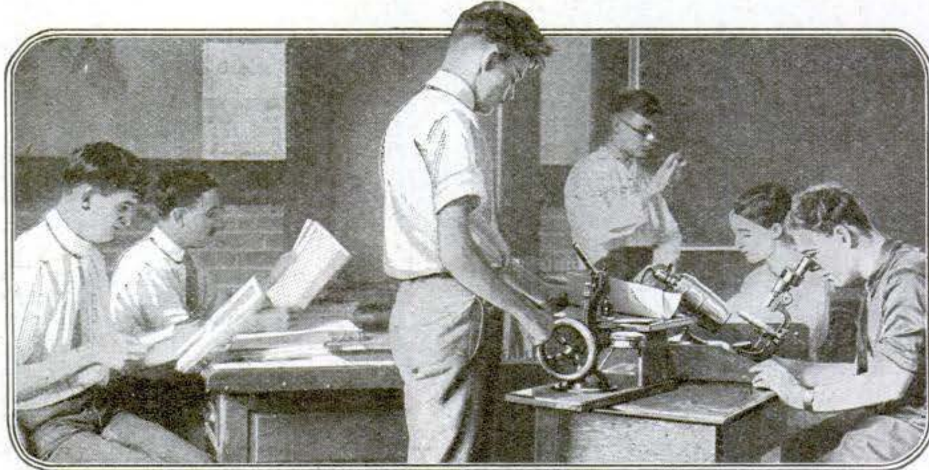
How paper is inspected and tested to see if it complies with standard specifications. The machine tests a sample for its bursting strength by registering the pressure in pounds per square inch required to break the paper. The man using the microscope is examining the fiber composition of the paper
