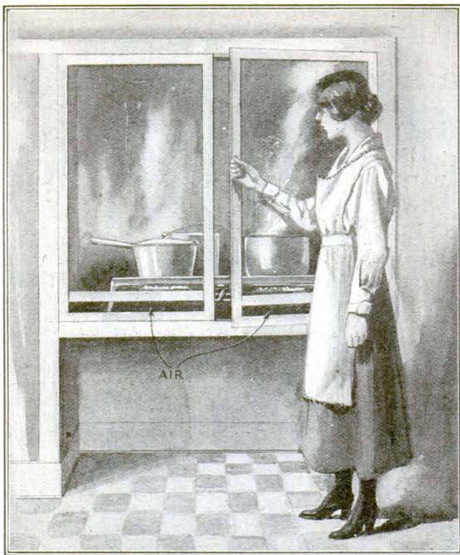
Chemists use a draught-closet when they work with compounds that give off nauseous or poisonous fumes. Now the draught-closet is used in the kitchen to carry off cooking odors
