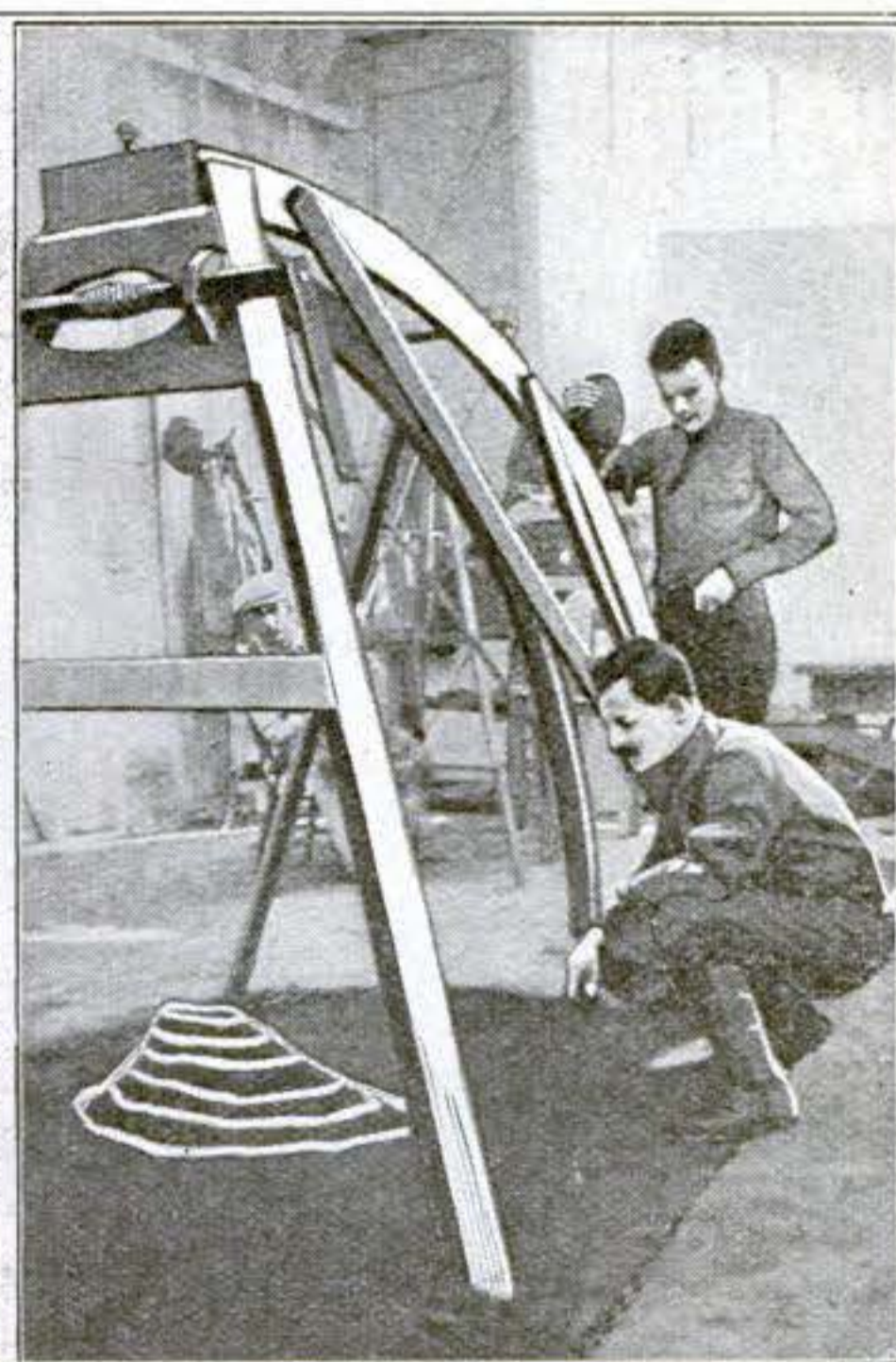
The curved track enables the camera to view the "mountain" as an airplane observer would
