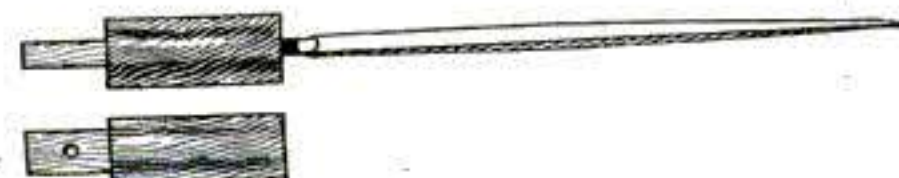
A three-cornered file mounted on a base, so that one corner can be used in marking the glass tube
