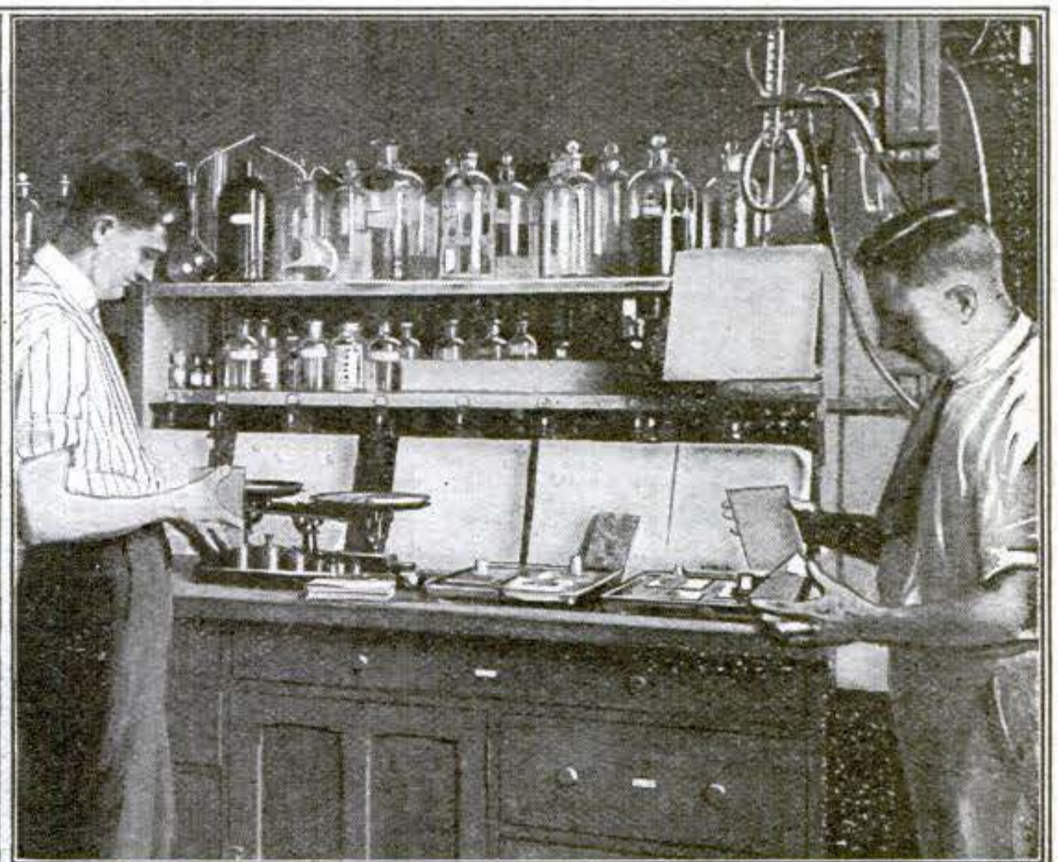
Testing wall-board by immersing it in water. A sample four by six inches is placed in water for six hours. Every hour it is weighed. An increase in weight of not more than 110 per cent means that it is a properly moisture-proof wall-board
