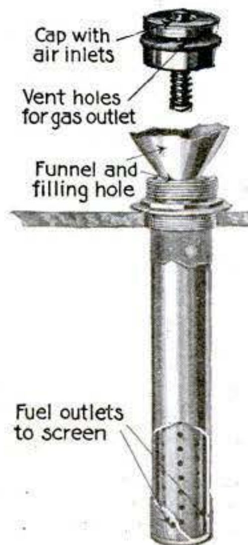
This innocent-looking tube takes the danger out of gasoline in several ways
