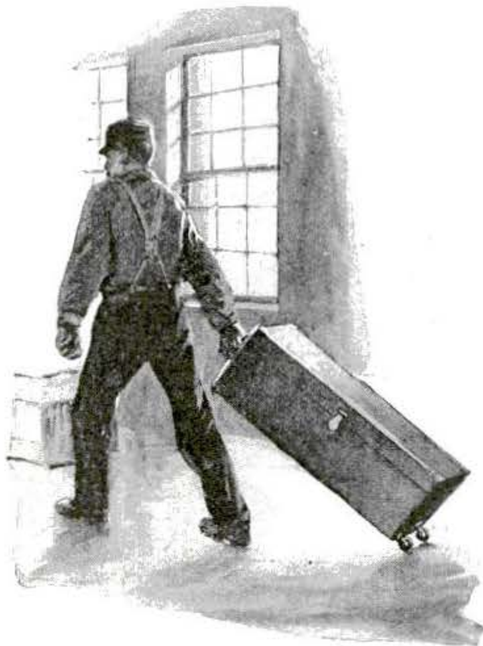
Casters on the end of a heavy tool box help to make the load much lighter
