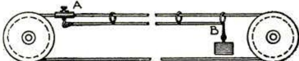
An extra line on the two pulleys for holding the smaller things for drying
