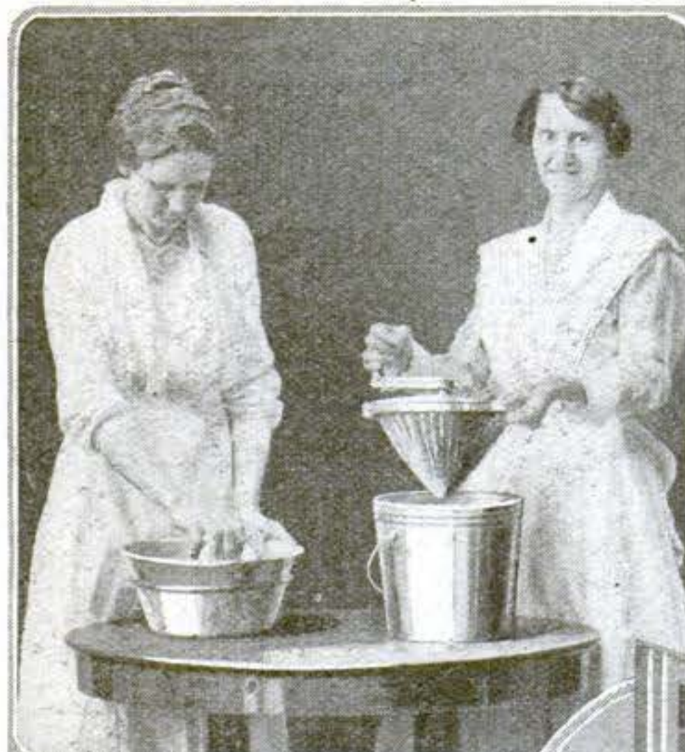
A cone-shaped colander with a hollow central column, which serves for a sleeve in the upper end of the handle. An inner grating shreds the food, forcing it through the perforations in the outer cone
