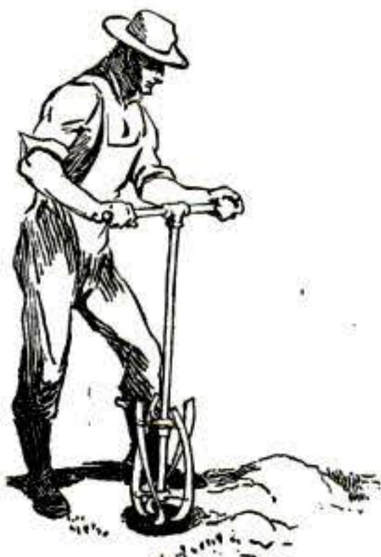
The blades of a lawn-mower used as a post-hole auger
