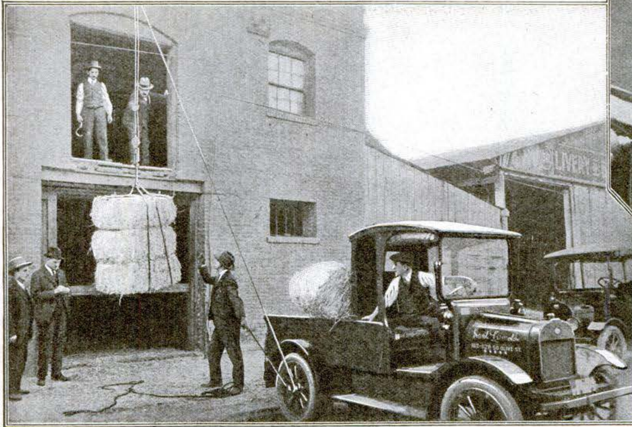
There seems to be no limit to the number of ways of utilizing an automobile. The truck in the picture above is jacked up in the rear and is used to hoist hay to the loft. The hub serves as the drum
