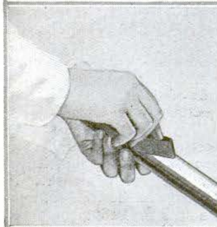
This metal-polisher looks like a pencil-eraser: it removes rust by merely rubbing the metal surface
