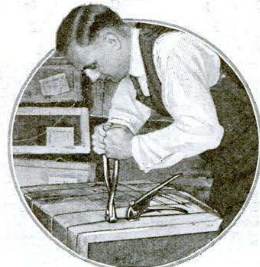
Tools that draw the strapping tightly around boxes, thus very effectually sealing them
