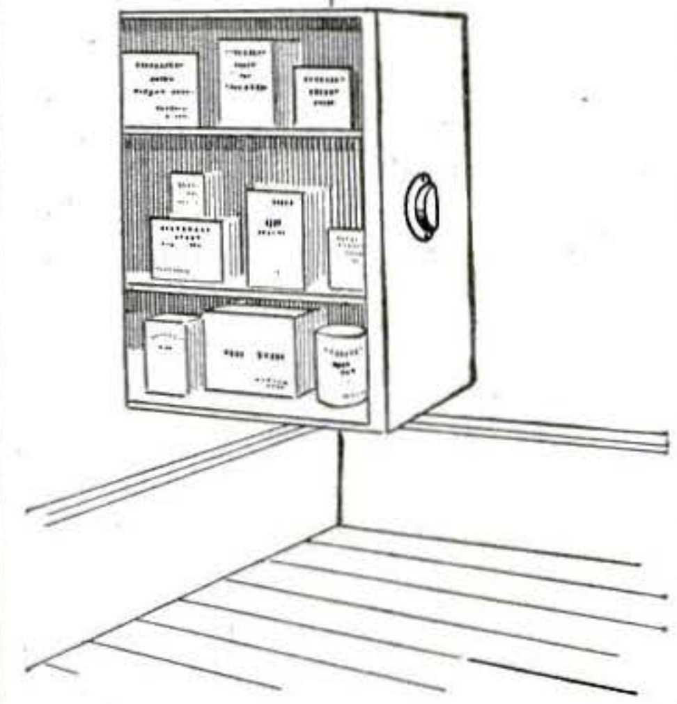
The drawer in an upright position as it is drawn from the wall
