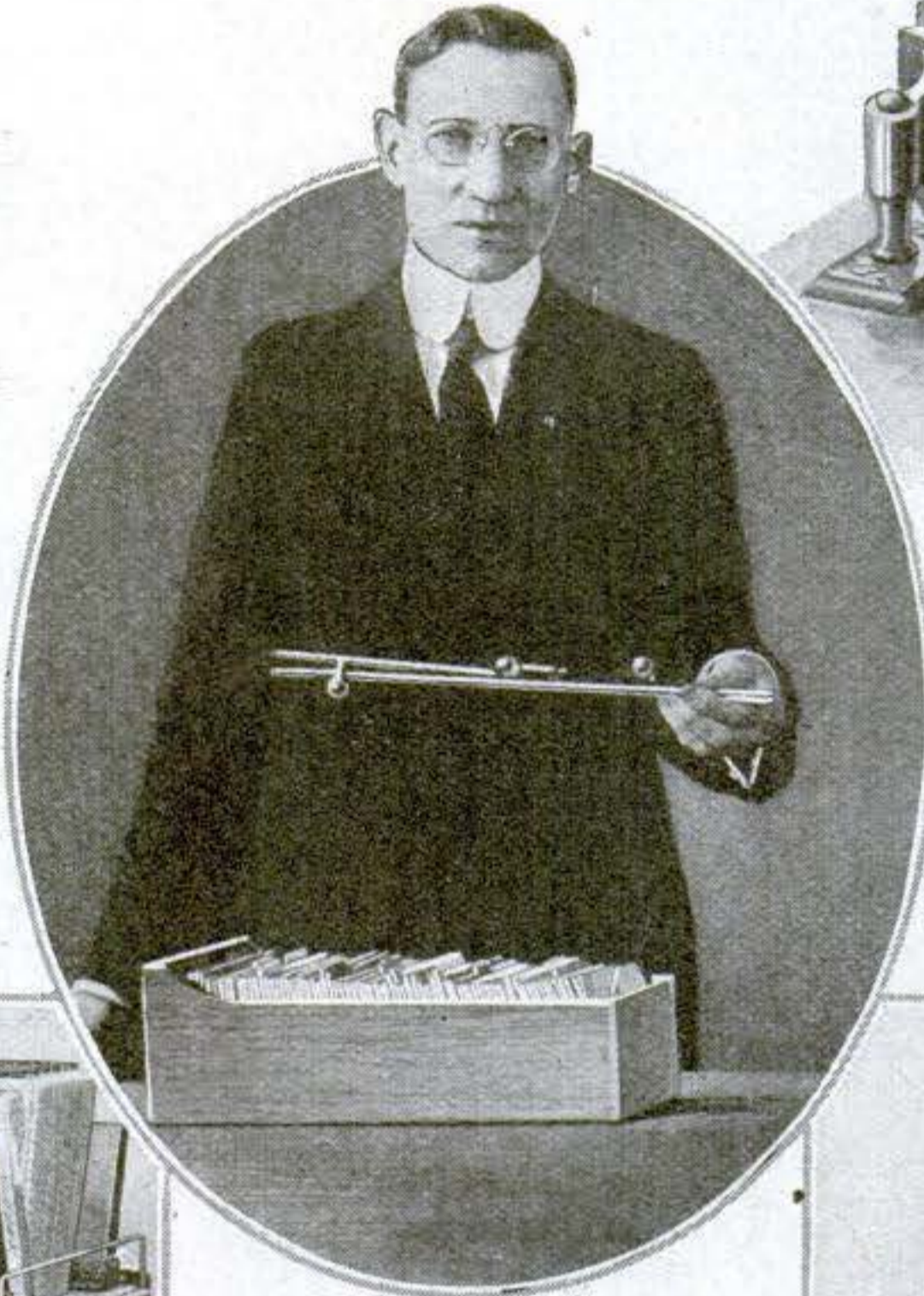
When a card is taken from the tray, the retaining attachment holds the location open
