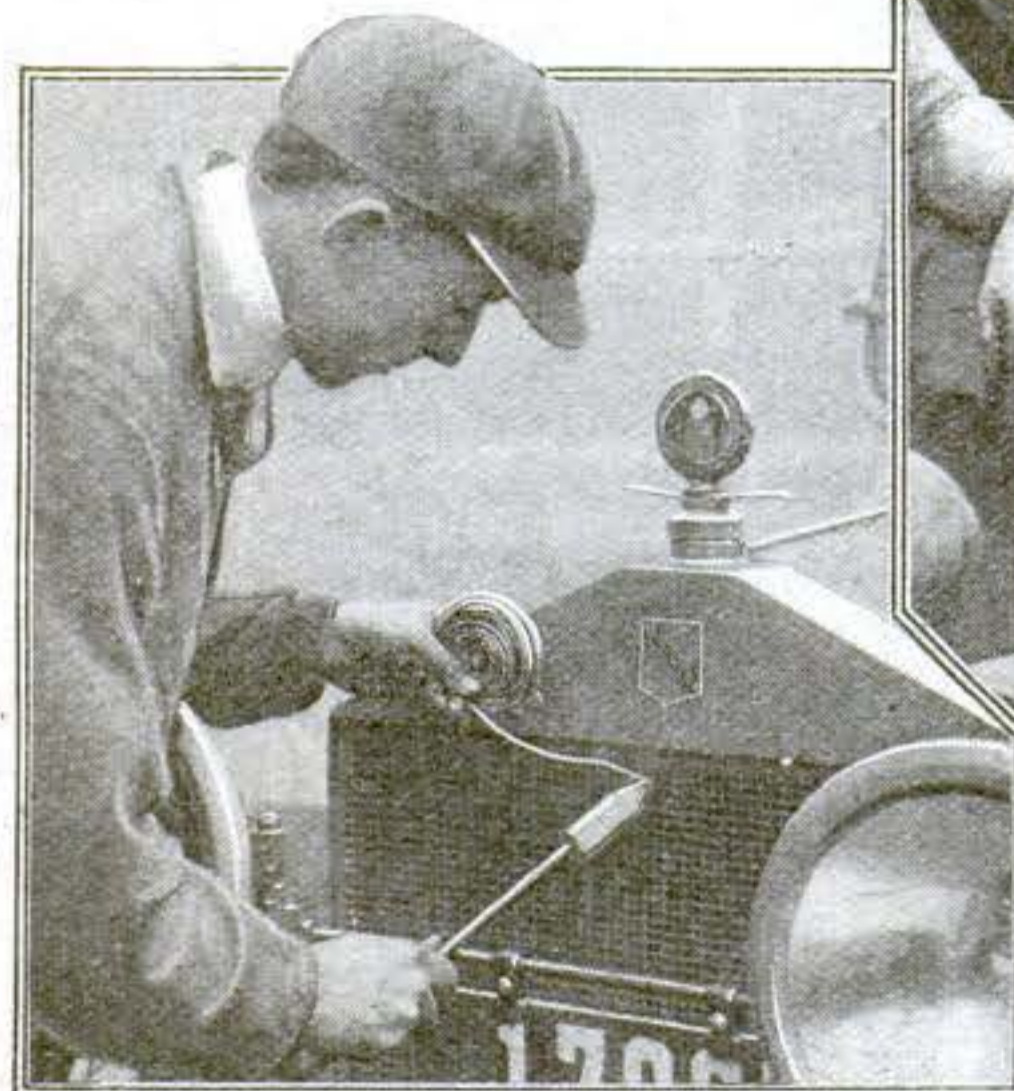
A new kind of solder comes in the form of a narrow tube with inside partitions containing an acid flux
